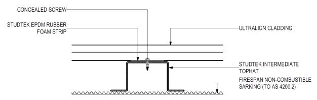
ULTRALIGN installation details are available in PDF and CAD on request. The ULTRALIGN installation details are provided for conceptual purposes only. These are not the only methods that can be used to attach ULTRALIGN, nor can they be used generically without consideration for each individual application. Good design engineering may preclude the choice of details used.
