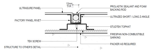
ULTRASURE installation details are available in PDF and CAD on request. The ULTRASURE installation details are provided for conceptual purposes only. These are not the only methods that can be used to attach ULTRASURE, nor can they be used generically without consideration for each individual application. Good design engineering may preclude the choice of details used.
