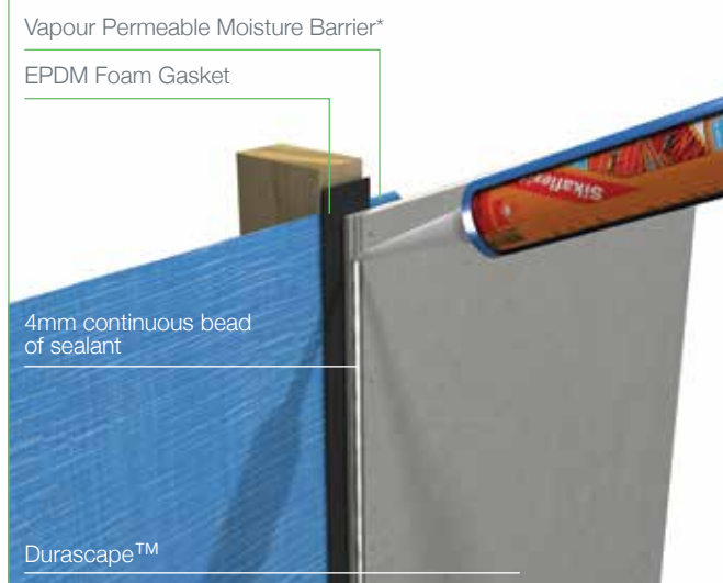
Figure 10 Apply Sealant
