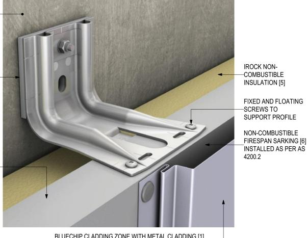
BLUECHIP CLADDING ZONE WITH METAL CLADDING [1], NATURAL CLADDING [2] OR TIMBER CLADDING [3] ON-STUDEK TOPHATS [4] (SEE SEPERATE DETAILS)
