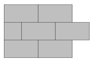
• Cutting should be carried out by using a fine-toothed saw or with a sharp knife ensuring accurate trimming to achieve close-butting joints and continuity of insulation.
