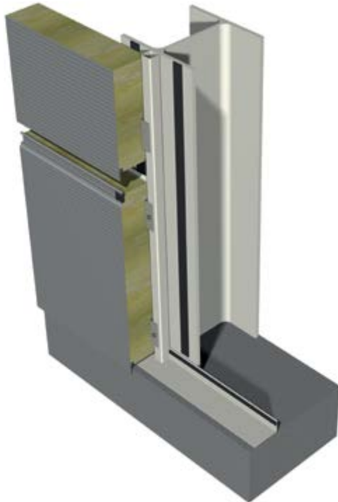
Fig. 34: Indirectly fixing back steel sheet into spacer
