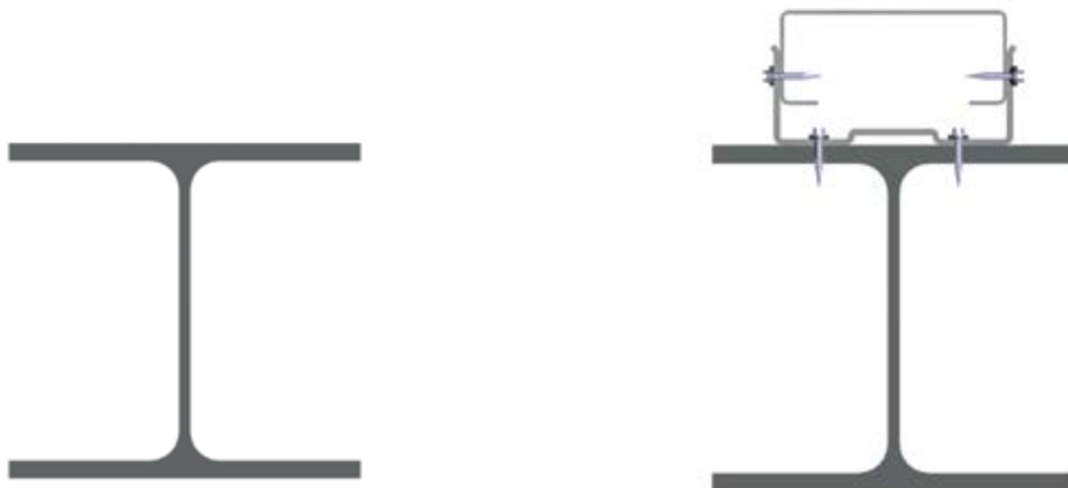
Fig. 21: Steel structure and steel structure with levelling sub-structure.
